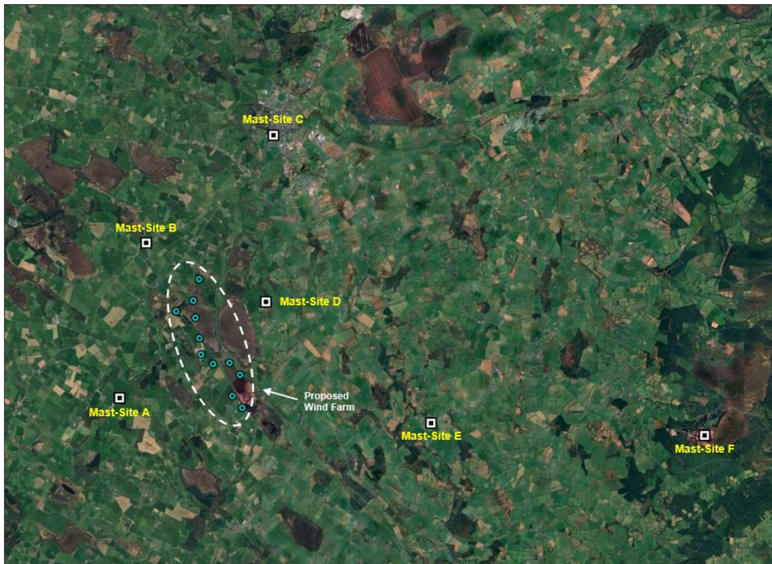
Figure 4. Telecom Mast-Sites Surveyed.
