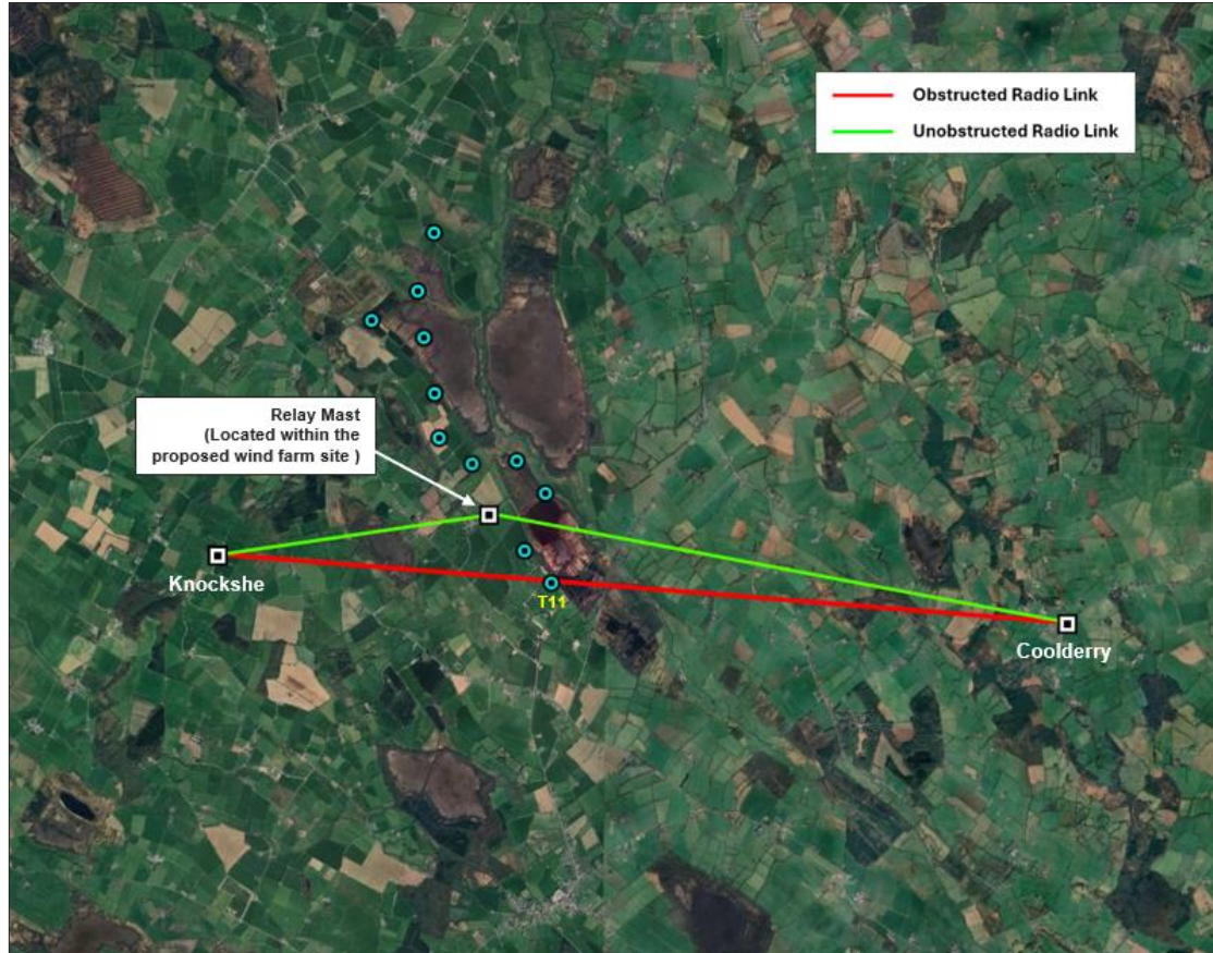
Figure 12. Proposed Relay Mast Location
