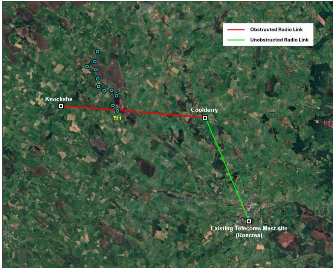
Figure 13. Re-routing via an alternative Eir Mast-site
