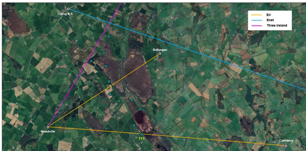
Figure 14. Plan View of Radio links in vicinity of proposed wind farm.
