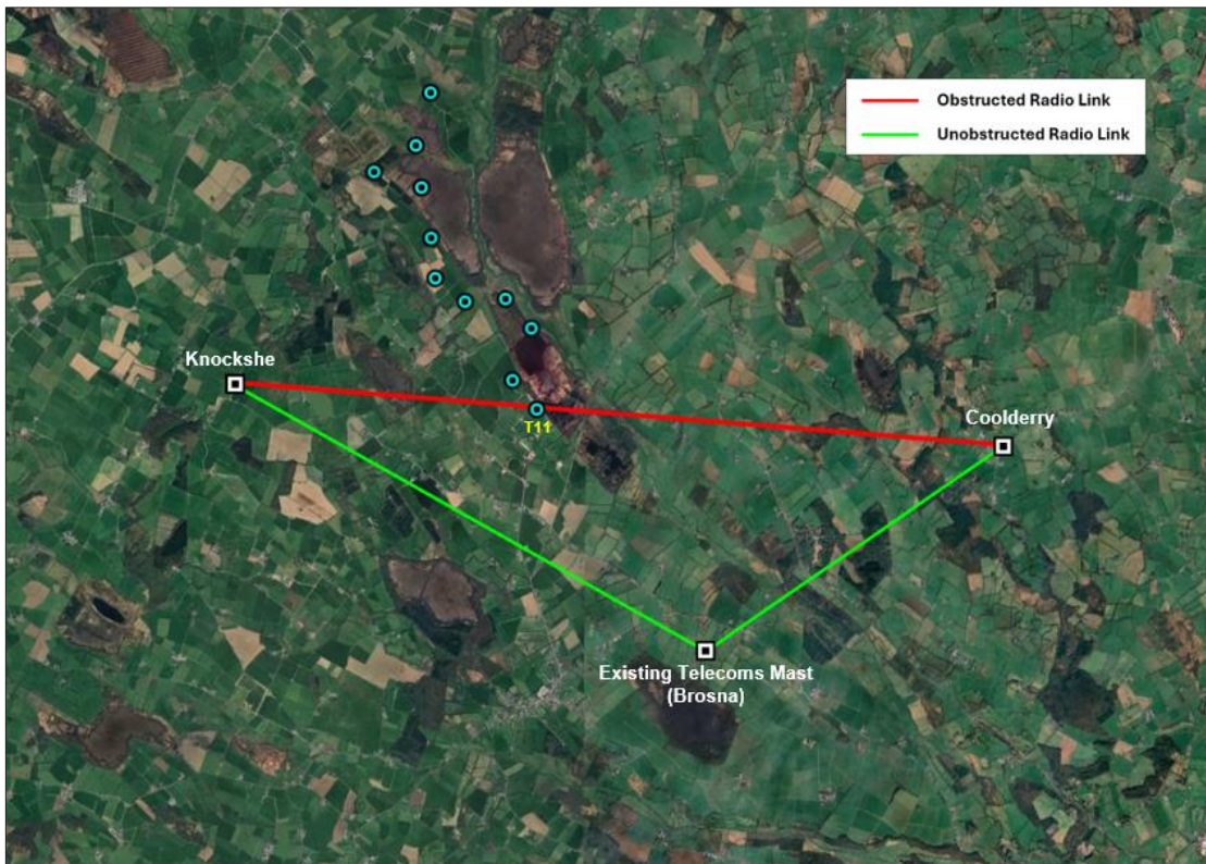
Figure 11. Relaying via Existing Eir Mast Site
